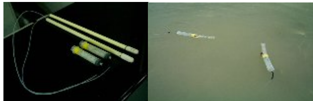
Gambar 3. Alat pengambil air antara ( porewater ) di sedimen terdiri dari pipa penyaring dan syringe . Figure 3. Instrument for porewater such as filter pipe and syringe.
